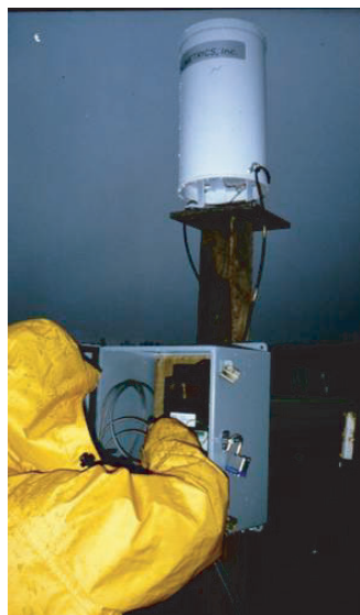
Figure 6.20 Tipping bucket rain gauge with data logger.
