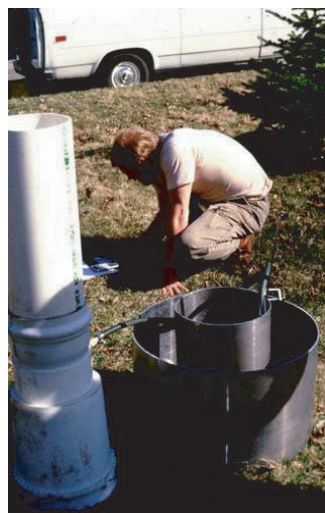
Figure 6.31 Double-ring infiltrometer measurements in disturbed urban soils in Oconomowac, WI.
