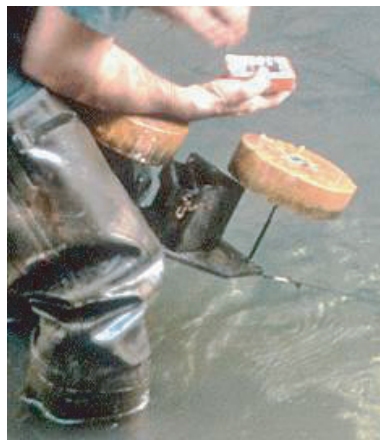
Figure 6.121 Diatometer for artificial substrate periphyton sampling.
