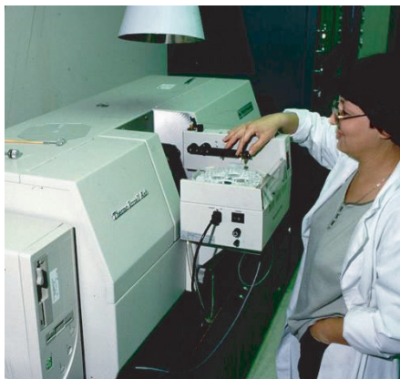
Figure E.10 Graphite furnace AAS used for stormwater analyses at the University of Alabama at Birmingham.
