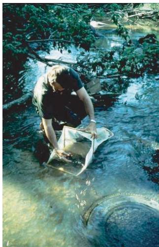
Figure 4.7 Natural substrate sampling using a Surber sampler in Coyote Creek.
