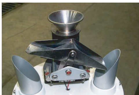
Figure 6.21 Close-up of tipping bucket rain gauge mechanism.
