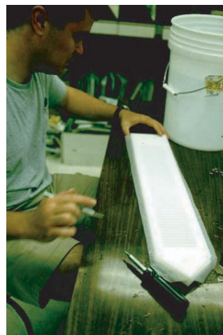
Figure 5.81 Small-volume peeper assembly showing 75-mm nylon screening.
