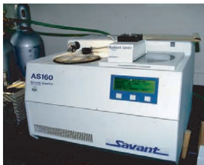
Figure E.20 Automatic vacuum/centrifuge concentrator (Savant AS 160).
