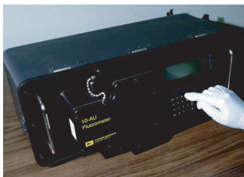
Figure 6.10 Current model Turner 10-AU fluorometer being calibrated in the laboratory before field deployment.
