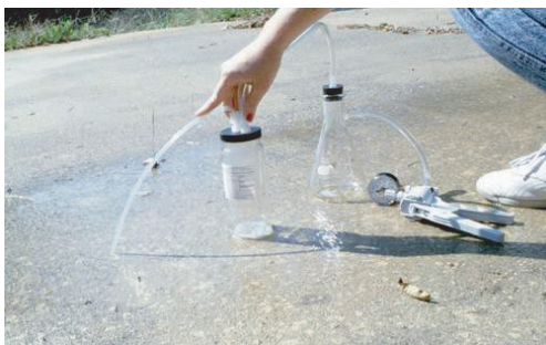
Figure 5.47 .Sheetflow sampler operated by hand vacuum pump.
