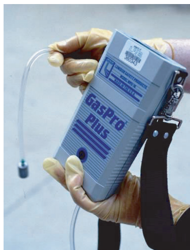
Figure 6.114 Portable gas analyzer for H 2 S and explosive conditions.
