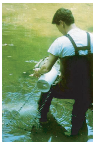
Figure 4.49 Placement of in situ pathogen die-off test chambers in Five-Mile Creek. (Courtesy of John Easton.)
