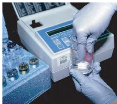
Figure 6.93 HACH AccuVac fluoride method.
