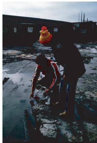
Figure 5.48 Sheetflow sampler being used to sample snowmelt.
