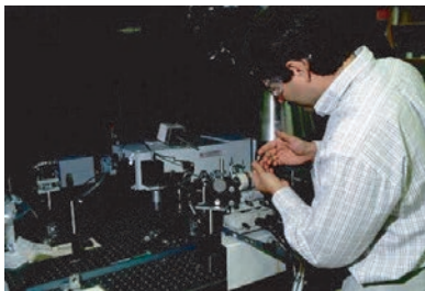
Figure 6.81 ° Laser fluorescence analysis of heavy metals being adapted for field analyses by UAB Physics Department.
