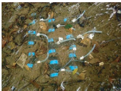
Figure 6.166 In situ sediment–water interface chambers buried.
