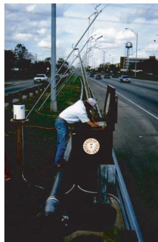
Figure 5.55 Sampler and rain gauge location at Austin freeway washoff test site.
