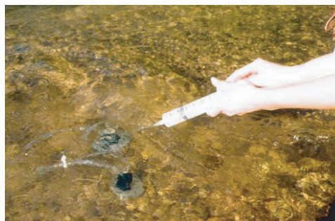
Figure 5.85 Withdrawing interstitial water sample from large-volume peeper.
