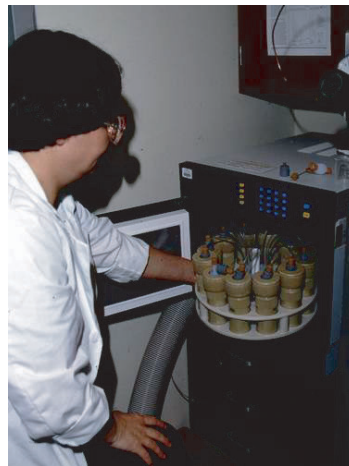
Figure E.13 Microwave digestion of stormwater samples for heavy metal analyses.
