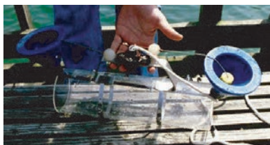
Figure 5.35 .Horizontal water sampler in open position before use.
