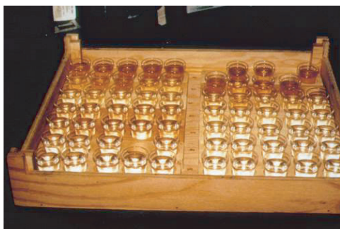
Figure 6.143 Test setup for the C. dubia short-term chronic toxicity test.
