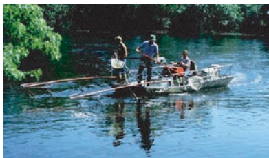
Figure 6.131 Boat electrofishing unit. (Courtesy of Wisconsin Department of Natural Resources.)
