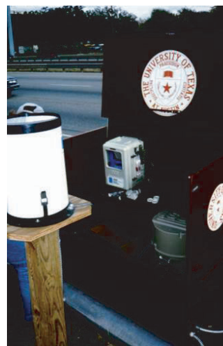
Figure 5.56. Sampler and flow monitoring equipment at Austin freeway washoff test site.
