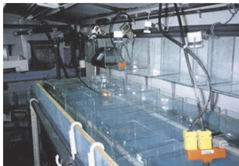
Figure 3.5 Lincoln Creek side-stream fish bioassay test facilities nearing completion.
