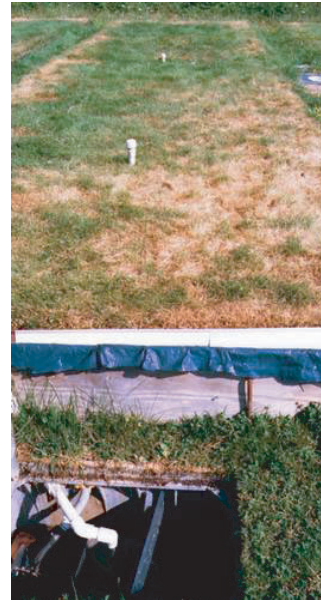
Figure 6.34 Soil infiltration test plot at University of Washington, Seattle.
