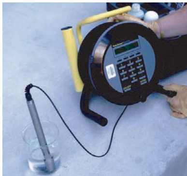
Figure 6.66 Petrosense being calibrated.
