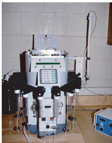
Figure E.24 OI GPC used to clean sediment extracts.
