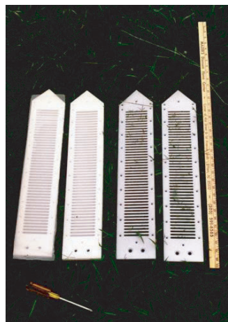
Figure 5.80 Disassembled small-volume, high-resolution peepers.
