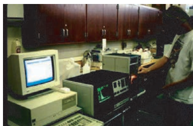
Figure 6.102 3Coulter Multisizer for stormwater particle size analyses.
