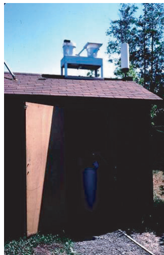
Figure 5.58 Wet-dry atmospheric deposition sampler in Bellevue, WA.
