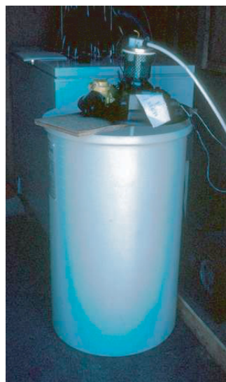
Figure 5.23 .Automatic sampler with large base for monitoring wide range of flows, with large chest freezer USGS discrete sampler in background, at Bellevue, WA.
