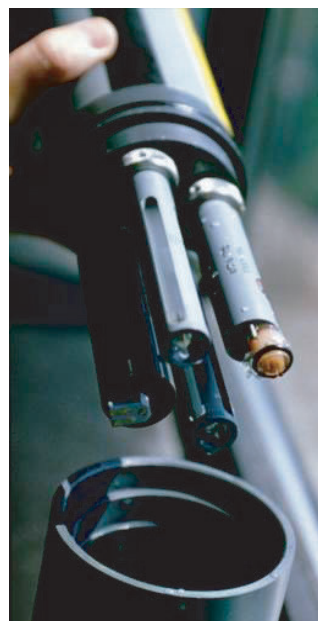
Figure 6.69 YSI 6000 sonde detail showing several probes.
