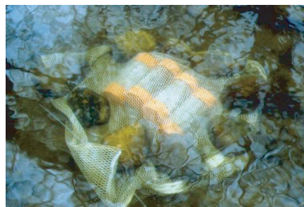
Figure 6.167 In situ chambers optimized for surface water and photoinduced toxicity effects from PAHs and UV light.
