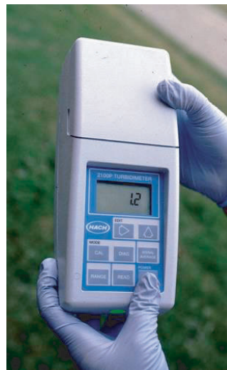
Figure 6.61 HACH turbidity reading.
