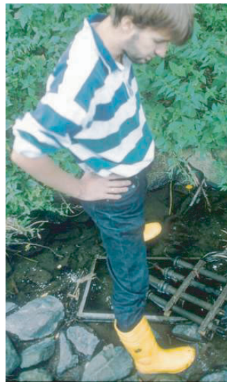
Figure 5.28 In-stream continuous probes at Dortmund, Germany, CSO monitoring site.
