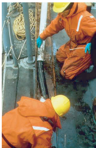
Figure 5.76 Emptying vibratory corer.
