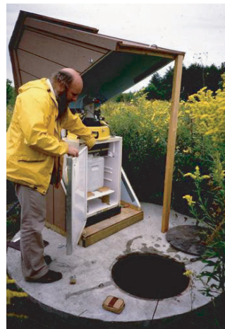
Figure 5.19 Refrigerated automatic sampler located at detention pond outfall in Madison, WI.
