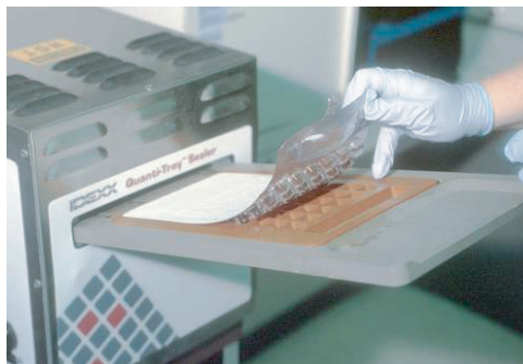
Figure 6.72 Placing analytical tray into heat sealing unit.
