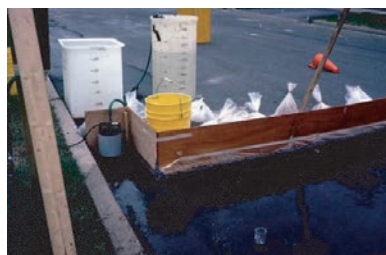
Figure 5.53. Runoff collection area for Toronto washoff tests.
