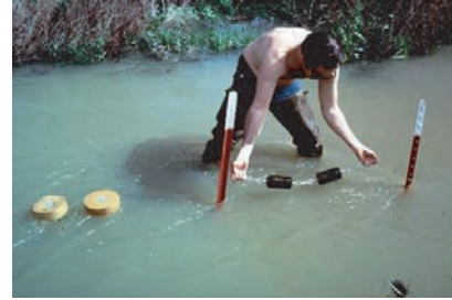
Figure 6.127 Periphyton sampler in place, plus Hester-Dendy samplers.
