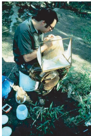
Figure 4.8 Removing benthic macroinvertebrate samples from Surber sampler.
