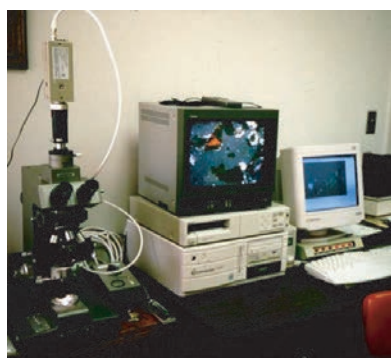
Figure 6.105 Microscope, video camera, and computer analyses of stormwater particles.
