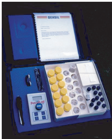
Figure 6.75 PetroFlag kit for field analyses of BTEX.
